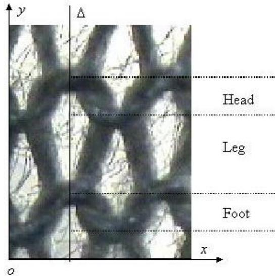
**Figure 1. Plain knitted fabric observed with optical microscope**
