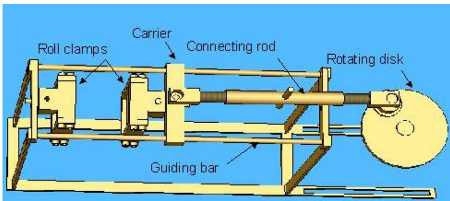
**Figure 7. Fatigue tester**
