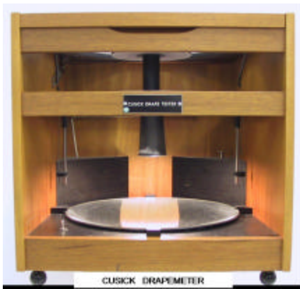
Figure 1: (a) Front view of Cusick Drapemeter, (b) Draped configuration of fabric
