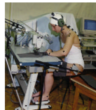
Figure 3: Bodily posture with marks in the course of sewing the second segment of the seam
