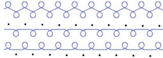
**Figure 2: Double woven rib knitted with blend of spun yarns**
