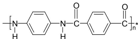
**Figure 1: Chemical structure of PPTA fibers**
