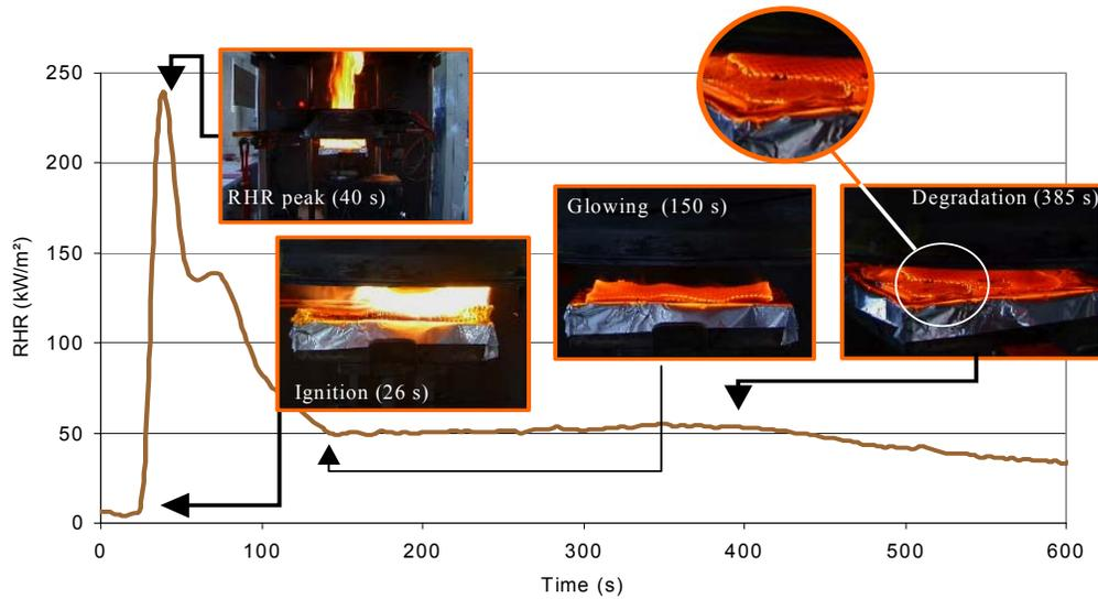
**Figure 6: Rate of Heat Release (RHR) curve of Kevlar at 75 kW/m<sup>2</sup>**
