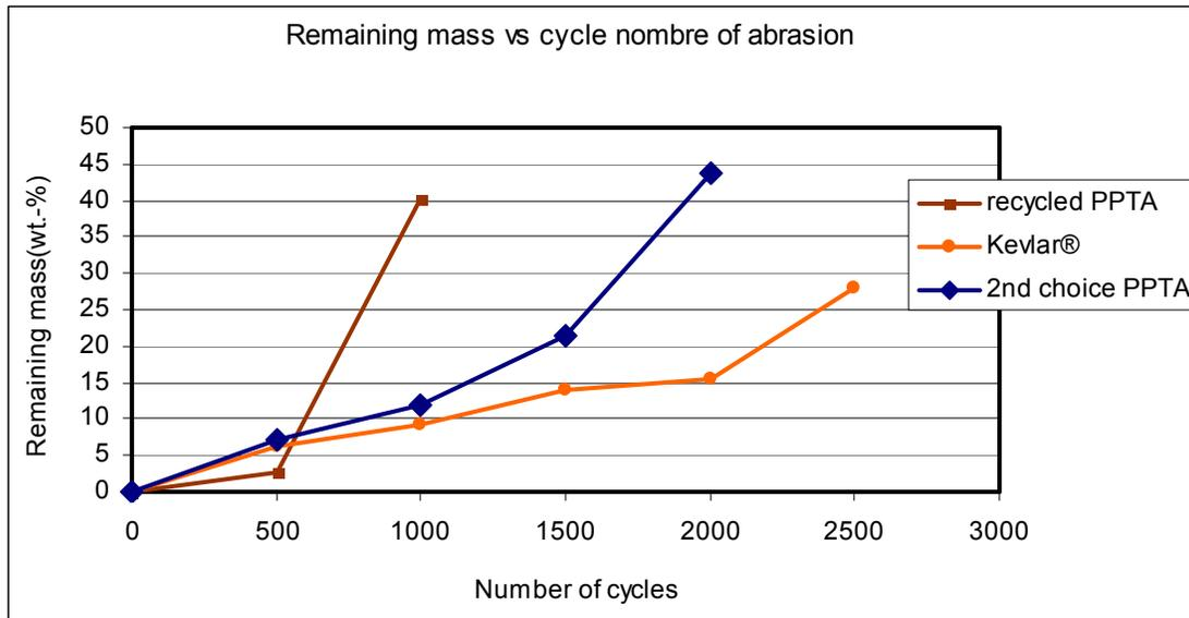
**Figure 5: Abrasion performances of the three PPTA fibers**
