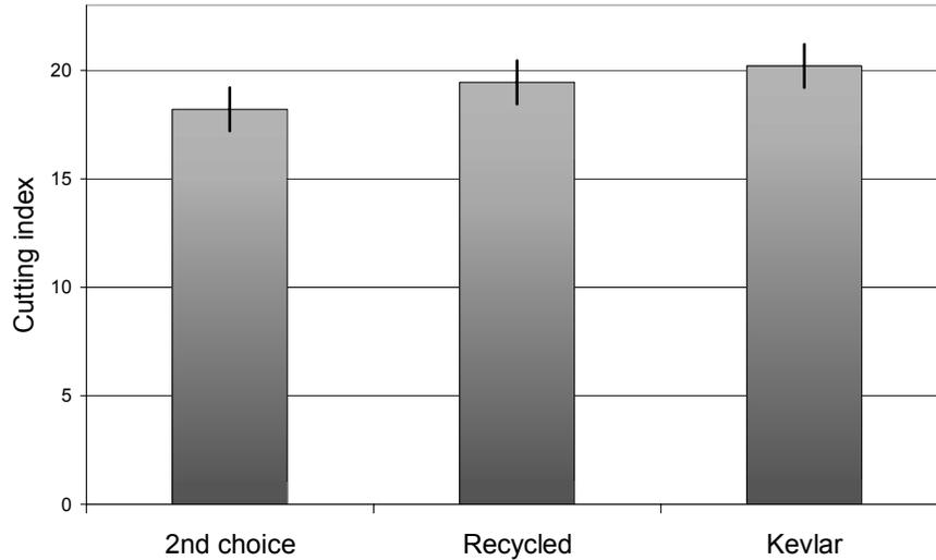
**Figure 4: cutting performances of the three PPTA fibers**
