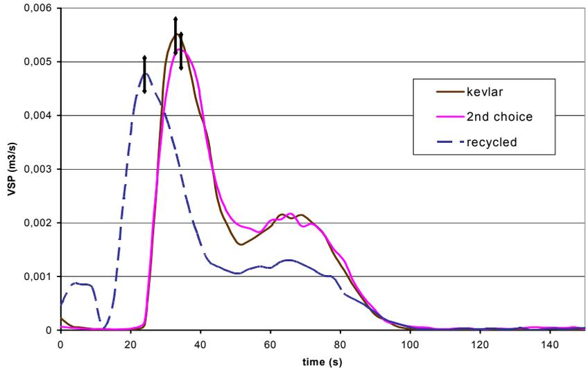
**Figure 10: VSP (Volume of smoke production) curves of the three PPTA fibers (external heat flux = 75 kW/m<sup>2</sup>)**
