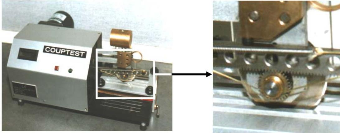
Figure 3: pictures of the cutting apparatus "Couptest"
