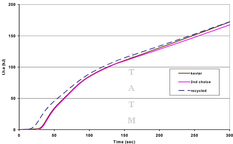
**Figure 9 :T.H.E. curves of the three PPTA fibers (external heat flux = 75 kW/m<sup>2</sup>)**
