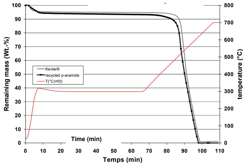
**Figure 11: Thermal treatment by TGA of recycled PPTA fibers and Kevlar**
