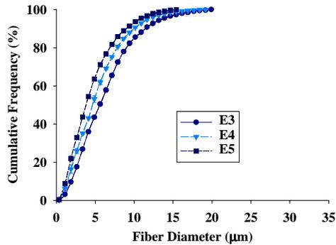
Figure 16. Cumulative frequency distribution of fiber diameters at different die temperature;  $9.6 \times 10^{-2}$  g/min/hole polymer throughput rate; 1.4 bar attenuating air pressure, and 327 °C attenuating air temp.; E3: 260 °C; E4: 293 °C; and E5: 327 °C die temperature.
