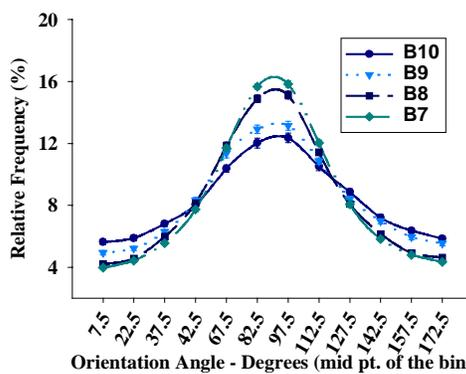
Figure 9. ODF for MB PP fabrics at different DCD;  $7 \times 10^{-2}$  g/min/hole polymer throughput rate, 1.4 bar attenuating air pressure, 21 m/min take-up speed, and 282 °C air temp.; B7: 14 cm; B8: 21 cm; B9: 26 cm; and B10: 31 cm.
