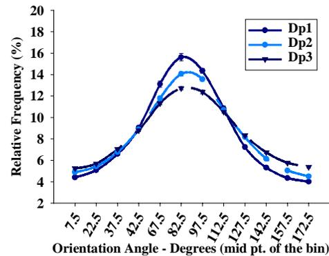
Figure 12. ODF for MB PP fabrics at different attenuating air pressures;  $9.6 \times 10^{-2}$  g/min/hole polymer throughput rate, 15 m/min take-up speed, 18 cm DCD, and  $282^\circ\text{C}$  air temp.; Dp1: 0.7 bar; Dp2: 1.4 bar, and Dp3: 2.1 bar.
