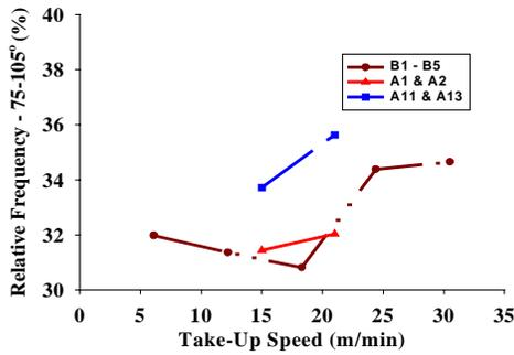
Figure 8. Maximum observed fiber fraction along “MD” for MB PP fabrics at different take-up speeds; 282 °C air temp.; B1-B5:  $7 \times 10^{-2}$  g/min/hole polymer throughput rate, 1.4 bar attenuating air pressure, and 14 cm DCD; A1 & A2:  $5.4 \times 10^{-2}$  g/min/hole polymer throughput rate, 1.4 bar attenuating air pressure, and 14 cm DCD; Ap11 & Ap13:  $5.4 \times 10^{-2}$  g/min/hole polymer throughput rate, 0.7 bar attenuating air pressure, and 18 cm DCD.
