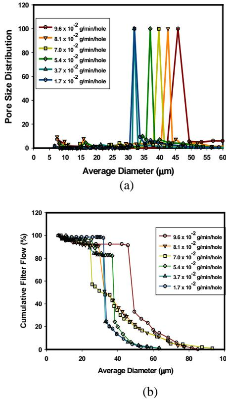
Figures 21 a & b. Pore Size Distribution and Cumulative Filter Flow (%) for MB PP Fabrics for variation in the Polymer Throughput (Take Up Speed: 20'/min., Number of Layers: 2, DCD: 15 cm, Air Pressure: 1.4 bar)
