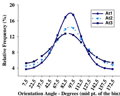
Figure 11. ODF for MB PP fabrics at different polymer throughput rate; 2.1 bar attenuating air pressure, 15 m/min take-up speed, 18 cm DCD, and  $282^\circ\text{C}$  air temp.; At1:  $5.4 \times 10^{-2}$  g/min/hole, At2:  $8.1 \times 10^{-2}$  g/min/hole, and At3:  $9.6 \times 10^{-2}$  g/min/hole.
