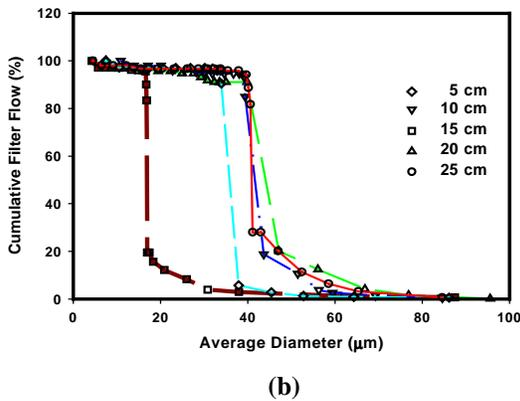
Figures 17 a & b. Pore Size Distribution and Cumulative Filter Flow (%) for MB PP Fabrics at different Die to Collector Distances. (Throughput :  $3.7 \times 10^{-2}$  g/min/hole, Air Pressure: 1.4 bar, Number of Layers: 2, Take Up Speed: 20 'min)
