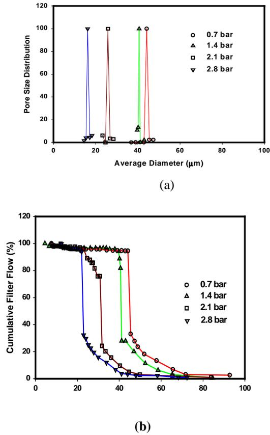
Figures 19 a & b. Pore Size Distribution and Cumulative Filter Flow(%) for MB PP Fabrics for variation in the attenuating air pressure. (Throughput :  $3.7 \times 10^{-2}$  g/min/hole, Number of Layers: 2, DCD 15 cm, Take Up Speed: 20 '/min)
