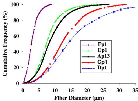
Figure 13. Cumulative frequency distribution of fiber diameters at different polymer throughput rates; 0.7 bar air pressure, 282 °C air temp., and 260 °C die temp.; Fp1:  $1.7 \times 10^{-2}$  g/min hole; Ep1:  $3.7 \times 10^{-2}$  g/min/hole; Ap13:  $5.4 \times 10^{-2}$  g/min/hole; Cp1:  $8.1 \times 10^{-2}$  g/min/hole; and Dp1:  $9.6 \times 10^{-2}$  g/min/hole.
