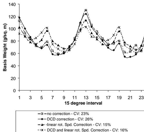
Figure 2. Two-Layer Basis-Weight Distribution Using the 2D Model
