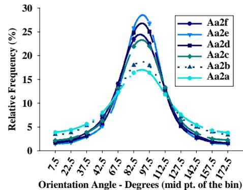
Figure 10. ODF for MB PP fabrics at different fiber-stream approach-angles;  $5.4 \times 10^{-2}$  g/min/hole polymer throughput rate, 1.4 bar attenuating air pressure, 21 m/min take-up speed, 14 cm DCD, and air temp. 305 °C; Aa2a: 90°; Aa2b: 79°; Aa2c: 61°; Aa2d: 46°; Aa2e: 36°; and Aa2f: 26°.
