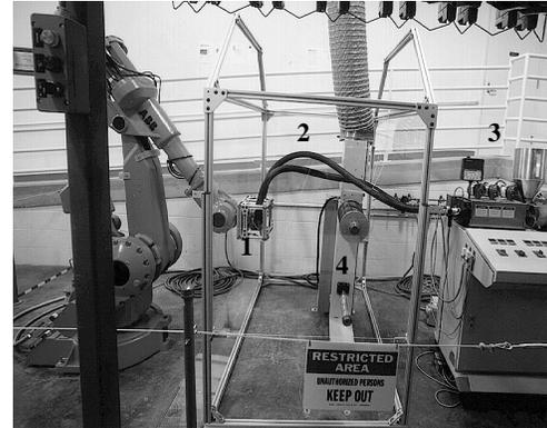
Figure 1. Robotic Fiber Assembly and Control System (RFACS)
