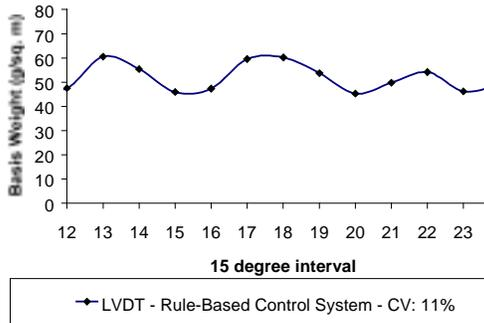
Figure 5. Rule-Based Control Results Using LVDT Feedback and 3D Triangularization
