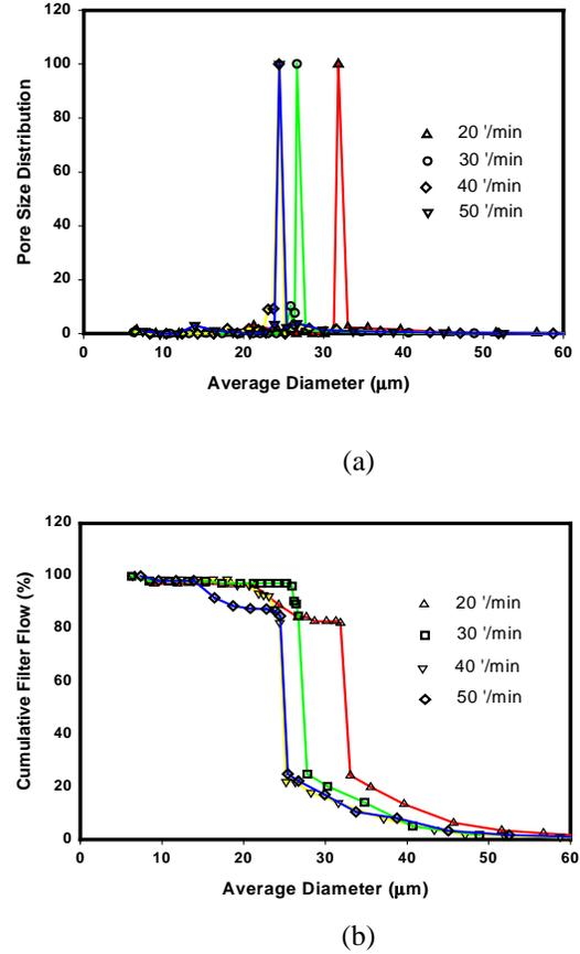
Figures 20 a & b. Pore Size Distribution and Cumulative Filter Flow(%) for MB PP Fabrics for variation in the web Take up Speed (Throughput :  $3.7 \times 10^{-2}$  g/min/hole, Number of Layers: 2, DCDC: 15 cm, Air Pressure: 1.4 bar)
