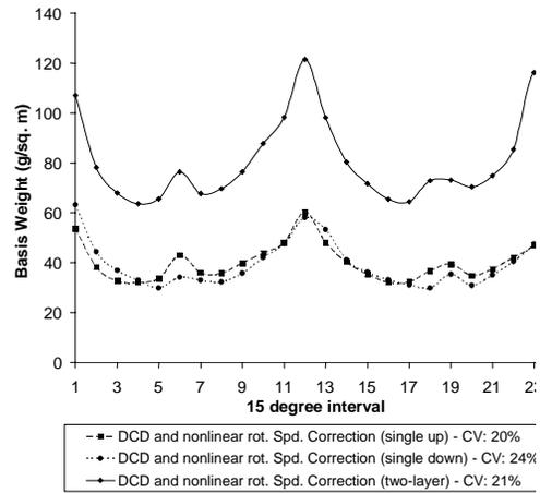
Figure 3. Single-Layer/Two-layer Basis-Weight Distribution using the 2D Model and Nonlinear Rotation Speeds
