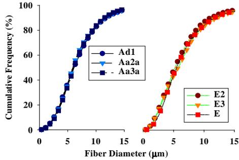
Figure 15. Cumulative frequency distribution of fiber diameters at different attenuating air temperatures;  $5.4 \times 10^{-2}$  g/min/hole throughput rate, 1.4 bar attenuating air pressure, and 260 °C die temp.: Ad1: 282 °C, Aa2a: 305 °C, and Aa3a: 327 °C;  $3.7 \times 10^{-2}$  g/min/hole throughput rate, 1.4 bar attenuating air pressure, and 260 °C die temp.: E: 282 °C, E2: 304 °C, and E3: 327 °C.
