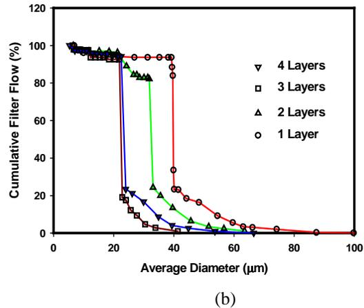
Figures 18 a & b. Pore Size Distribution and Cumulative Filter Flow (%) for MB PP Fabrics for variation in the number of layers. (Throughput :  $3.7 \times 10^{-2}$  g/min/hole, Air Pressure: 1.4 bar, DCD 15 cm, Take Up Speed: 20 'min)
