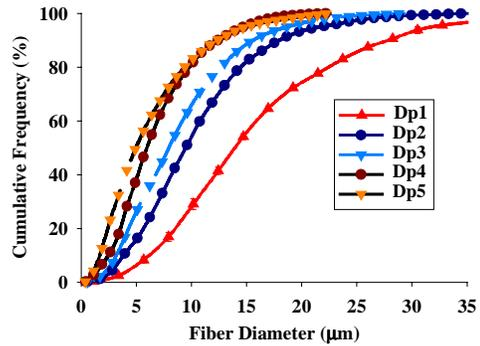
Figure 14. . Cumulative frequency distribution of fiber diameters at different attenuating air pressure;  $9.6 \times 10^{-2}$  g/min/hole throughput rate, 282 °C air temp., and 260 °C die temp.; Dp1: 0.7 bar; Dp2: 1.4 bar; Dp3: 2.1 bar; Dp4: 2.8 bar; and Dp5: 3.5 bar.
