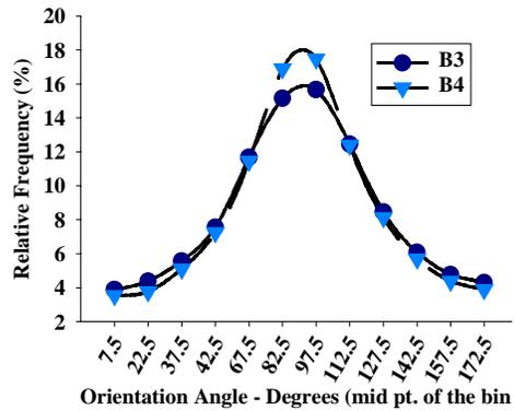
Figure 7. ODF for MB PP fabrics at different take-up speeds;  $7 \times 10^{-2}$  g/min/hole polymer throughput rate; 1.4 bar attenuating air pressure; 14 cm DCD and 282 °C air temp. ; B3: 18 m/min and B4: 24 m/min.
