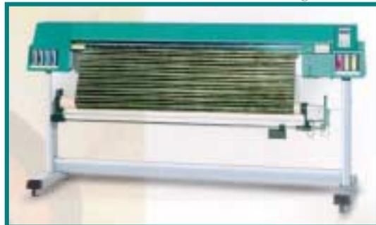
The continuous ink-jet method involves the use of a highly pressured, continuous stream of ink, which has been forced through a microscopic nozzle. Tiny drops are created from this stream by high frequency stimulation and directed to the desired location by a variable electric charge [21,22]. This technology allows relatively high-speed production of digitally printed fabric. Challenges still to be overcome include reducing
