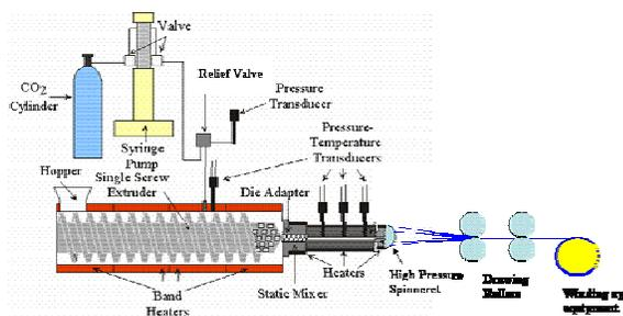
**Schematic for Supercritical Fluid Extrusion of Nanocellular Fibers**
