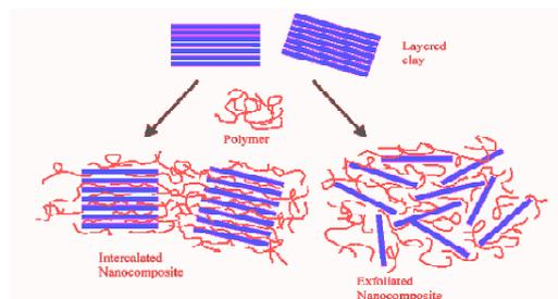
**Schematic of a nanosilicate composite**
