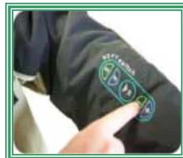
**Figure 1: Integrated Textile Keypad**
