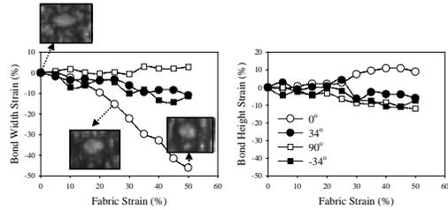
Figure 9: Unit cell strains along the cross (width) and machine (height) as functions of fabric tensile strain, applied at 0, +34, 90 and -34°
