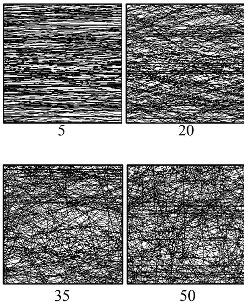
Figure 6. Images with varying degrees of anisotropy
