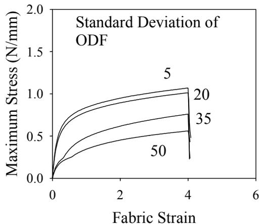
Figure 7. Web Stress-Strain curves as function of Anisotropy.
