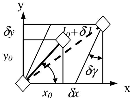
Figure 3. Incremental deformation of web
