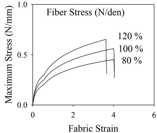
Figure 5. Web Stress-Strain curves as function of fiber strength
