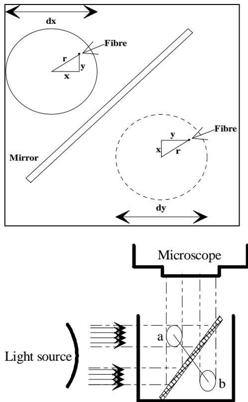
Figure 3: Modified Technique for Observing Two Orthogonal Projections of a Yarn [3] (a yarn, b image)
