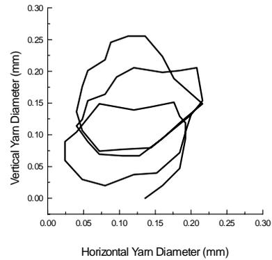
Figure 10: Tracer Fibre Configuration as Viewed from the Yarn Cross-section along the Yarn
