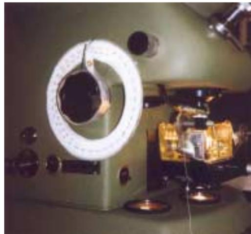
Figure 4: A Protractor Attached around Focusing Knob
