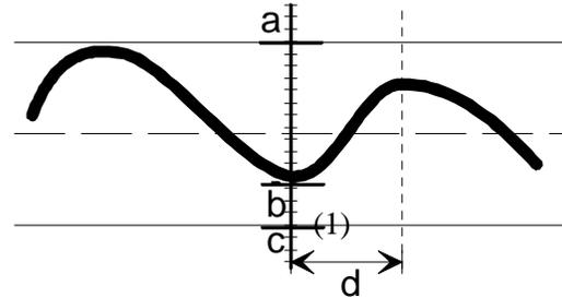
Figure 2. Measured Distances in a Yarn Containing Tracer Fibre
