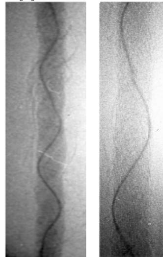
Figure 1: Tracer Fibres in Short Staple Yarns
