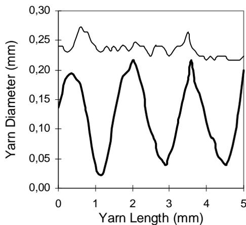
Figure 8: Observed 2-Dimensional Path of a Tracer Fibre in a Yarn. Note: The thin line indicates the correspondent yarn diameter fluctuation
