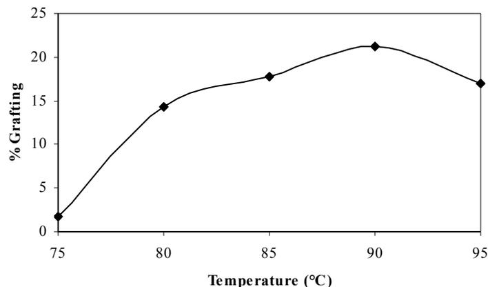
Fig.3 Variation of the grafting percentage versus temperature reaction ; [METAC]= 1.8 mole/l ; [initiator]=  $2 \times 10^{-2}$  ; time 2 hours.
