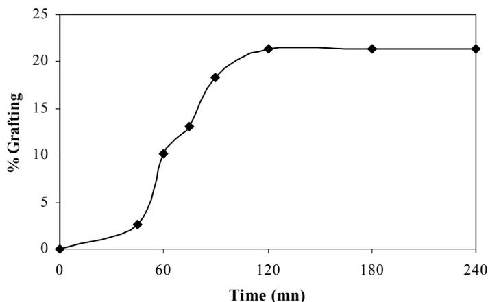
Fig.4 Variation of the grafting percentage versus time reaction ; [METAC]= 1.8 mole/l ; [initiator]=  $2 \times 10^{-2}$  ; temperature 90°C.
