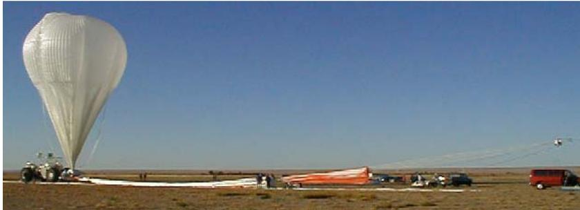
**Figure 2 Zero Pressure Balloon in Launch Configuration**
