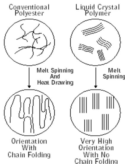
**Figure 5 Schematic of Molecular Chain Structure of Vectran Fiber**
