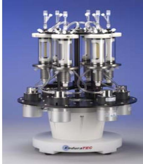
**Figure 8: Laboratory bioreactor for *in vitro* tissue engineering. Courtesy of Enduratec Inc.**
