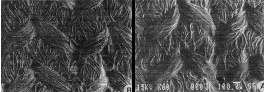
Figure 1: Knitted polyester vascular prosthesis with gelatin coating for improved
