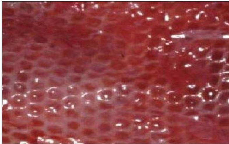
**Figure 12 : Porous warp knitted structure with stretch and recovery properties engineered to support the growth and proliferation of heart muscle cells seen after 6 months in a canine model.**
