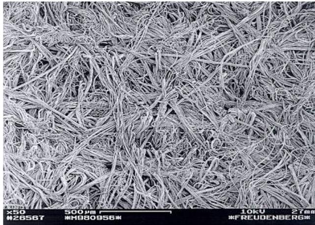
**Figure 11: Porous nonwoven structure fabricated from microdenier fibers.**
