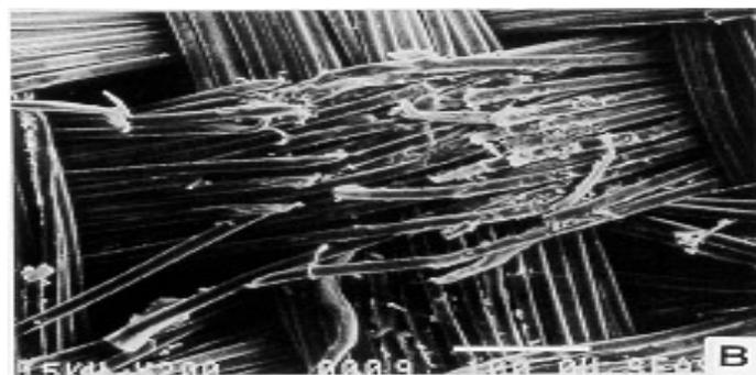
**Figure 3: Scanning electron micrograph of a woven polyester endovascular stent graft retrieved from the patient after 29 months *in vivo* showing evidence of surface abrasion.**
