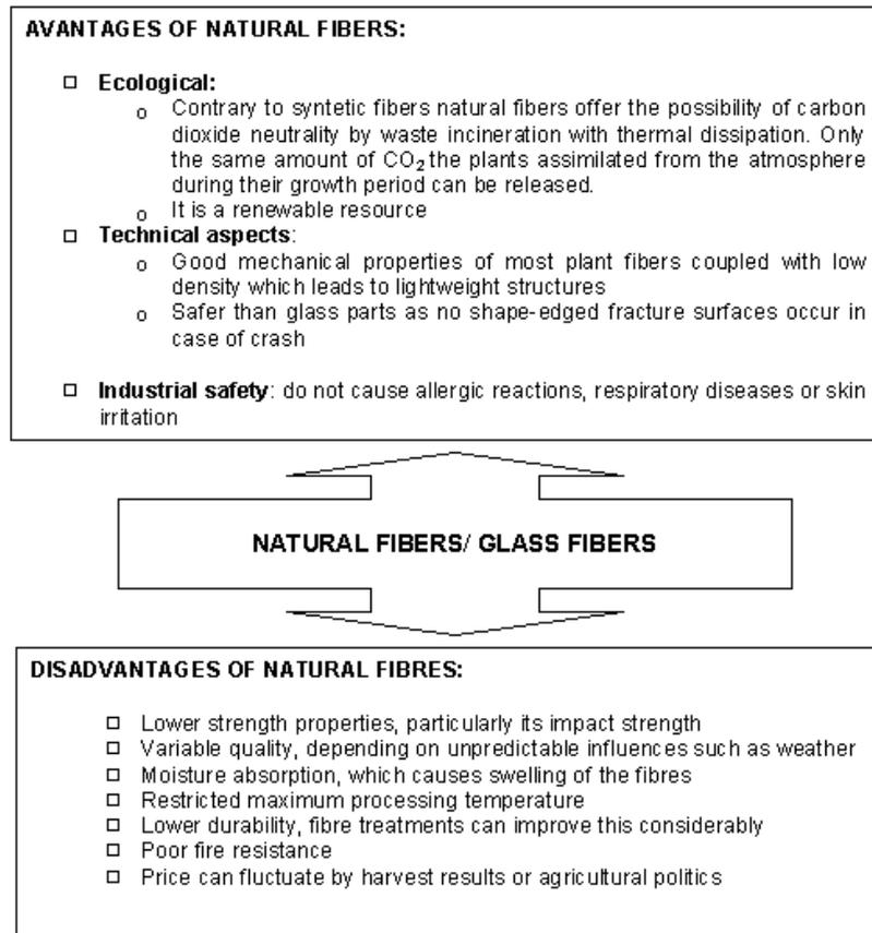
**Figure 1 Advantages/disadvantages of natural fibers used in automotive applications**
