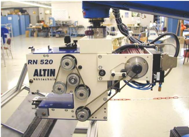
Fig. 2 Double Lock Stitch Head
