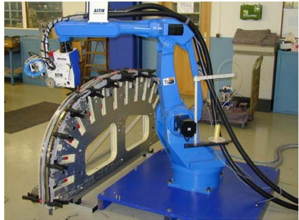
Fig. 11 Design of a Fixture for an Aircraft Structure
